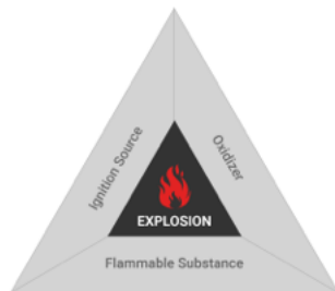
Figure 0: Three Required Elements for Occurrence of an Explosion
