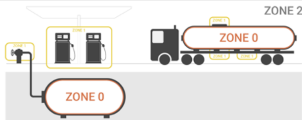
Figure 1: Zone Classification for Gas/Vapor/Mist
